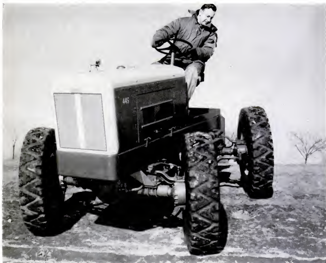
Four-wheel steering. Commercial version of an Army machine (PS, Dec. '57), this tractor can run sideways on four oblique wheels. Steering of the Napco Crab, controlled by knuckle joints, is done with front or back wheels. Front one way, rear the other, it turns in a 12-foot radius.
